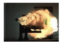
Next, an electric pulse is sent to the railgun, creating an electromagnetic force accelerating the projectile to Mach 7.5. Using its extreme speed on impact, the kinetic energy warhead eliminates the hazards of high explosives in the ship and unexploded ordnance on the battlefield.
